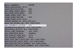
The EAS interface that communicates with the MC400 has the ability to engage what is known as a Macro. (The macro section is located at the bottom of this config file.) The EAS automatic action will trigger the macro to run the audio or any other needed action via that macro.
