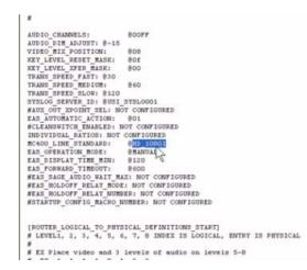
By the way, all possible formats are listed up above in the [remarked out] MC400 Line Standard sub-section (of this section).
