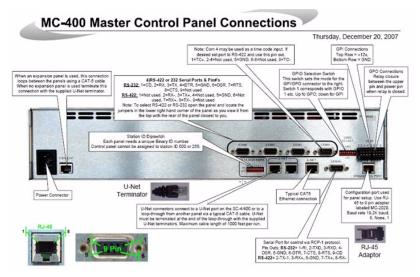
The four com ports (1 - 4) correspond to the above, non-remarked lines in the configuration file. The first line, given a default label of AVAILABLE\_PANEL, is designated for protocol.
