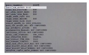
Set to a default of -15db, with a possible range of 0 to -45. This is used to dim the audio monitor output. Pressing the audio dim button will 'dim' the audio to that particular value.
