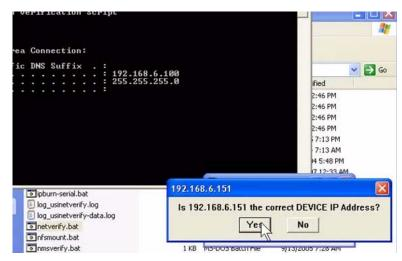
When you confirm, the system will ping the device, complete an NFS mount test (to make sure the NFS Server is running), then complete a system name check.
