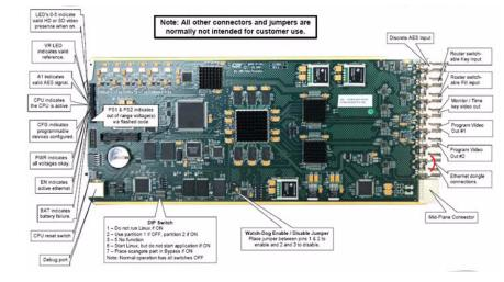
Note the BNC connectors along the card's right edge, as shown in the illustration. The top connector is labeled 'Discreet AES Input', and would correspond to the #7 connection if this card occupies the 0 - 7 slot, #15 in the next slot, #23 in the following slot, etc. The audio will enter through this BNC. The digitally converted EAS audio (becoming an AES stream) in plugged directly into this BNC. The configuration file will manage the remaining detail, playing the audio out as needed.
