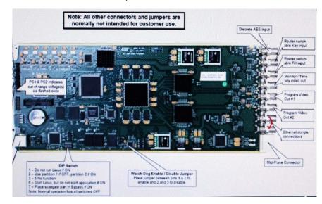
The first BNC is the Discreet AES Input and the second BNC is the external key input, while the third BNC is the external fill input. The next is the Preset, or master control system's monitor output, while the next two BNCs correspond to the Program video outputs. Finally the last two BNCs correspond to the Ethernet ports. These connectors require an Ethernet adapter that plugs onto these ports.
