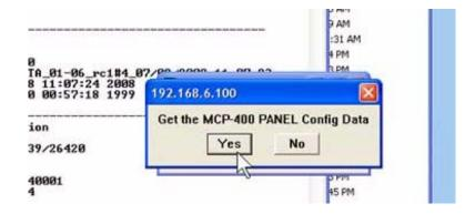
Next, re-launch Tera Term, enter the panel's IP address at the '...New Configuration' window, and type HD config at the command prompt.
