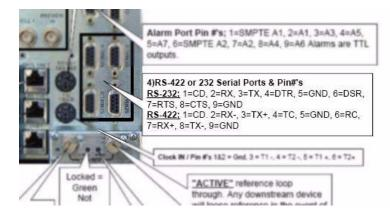
MC-2020 usage also requires jumper modification on the CPU card, to either 422 or 232 positioning. MC-400 usage involves lifting the MCP-2020's lid and moving the jumpers (inside) to either 422 or 232 positioning.
