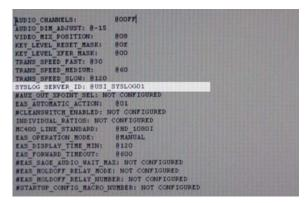
SYSLOG01 corresponds to the name that is assigned to the USI logging program. This is placed on the C drive after the install2020 is run (for that particular logging application). This allows the logging application (when it is running) to locate every channel that has this 'turned on'. The name on this line will match whatever happens to be in the USI logging.
