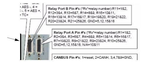
Port A contains 11 relays, while port B contains the remaining relays (up to 21). These ports are shown in the upper right corner of the illustration.
