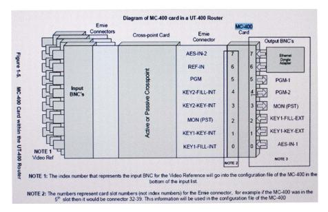
In this case the card occupies slot 0 - 7, and if the card were placed in the next slot, the outputs would become 8 - 15, and so on.
