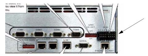
One of the power source's wires would attach to the relay matrix, while the other [side] of the power source attaches to the sending device – the device sending the pulse or latch to the GPI. The 5+ volt power source effectively energizes this opto. In the case of a GPO, both wires simply attach the chosen relay to the device that is receiving the pulse or latch.
