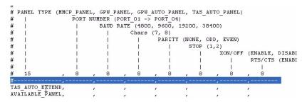
This line will always indicate the exact number of spaces needed between each comma, and the line immediately above this one shows the actual number of spaces required in the line. This format is important and must be followed exactly.
