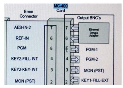
If for example, there were two additional keys that needed to be used besides the external key (note the output BNCs), there are two internal keyers along the Ernie connector block (illustration) utilizing the input ports 0 and 1, and 3 and 4 respectively.
