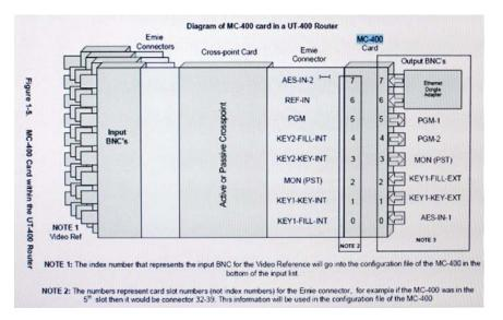
The detail beneath 'Ernie Connector' (to the left of above) represents the connector that is internal to the router. This is essentially the connective hardware between the MC-400 card, the Crosspoint card, and the Input BNCs where the Sources enter.
