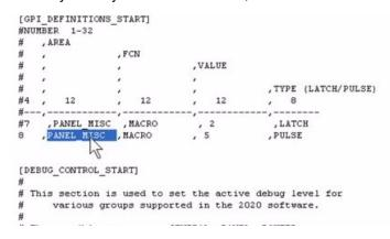
This name would typically correspond to this particular button's action. Keep in mind that there are only three types of GPI's applicable to this function; a take, preroll, or macro. In our example the existing type is a macro, and the associated value number (in the next column) is derived from the 'Macro Definitions Start' table (above).
