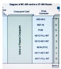
The router's inputs are processed through the Ernie connectors, sent through the crosspoint card, then directed to MC-400 card as program and preset outputs. The *Reference In* corresponds to the master control's format type, either SD or HD. This signal is also processed through the Ernie connector.
