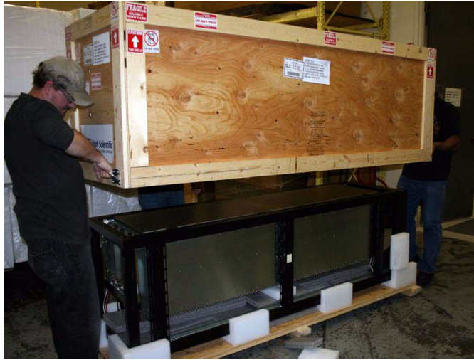
FIGURE 2-8. Carton housing lifted from base - 2
