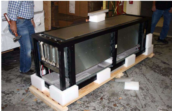
FIGURE 2-9. Carton housing separated from base
