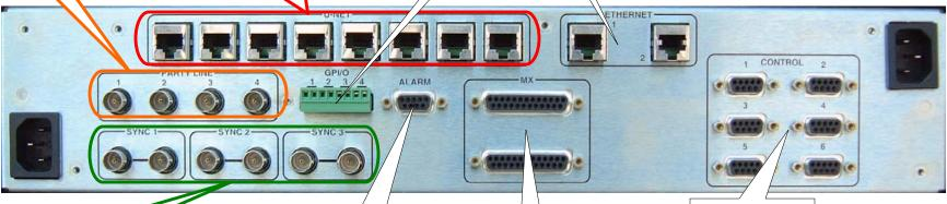
A maximum of 3 sync sources may be connected to the loop thru Sync Connectors. Sync source must be analog black burst or analog tri-level sync. DO NOT connect SDI reference signals.
