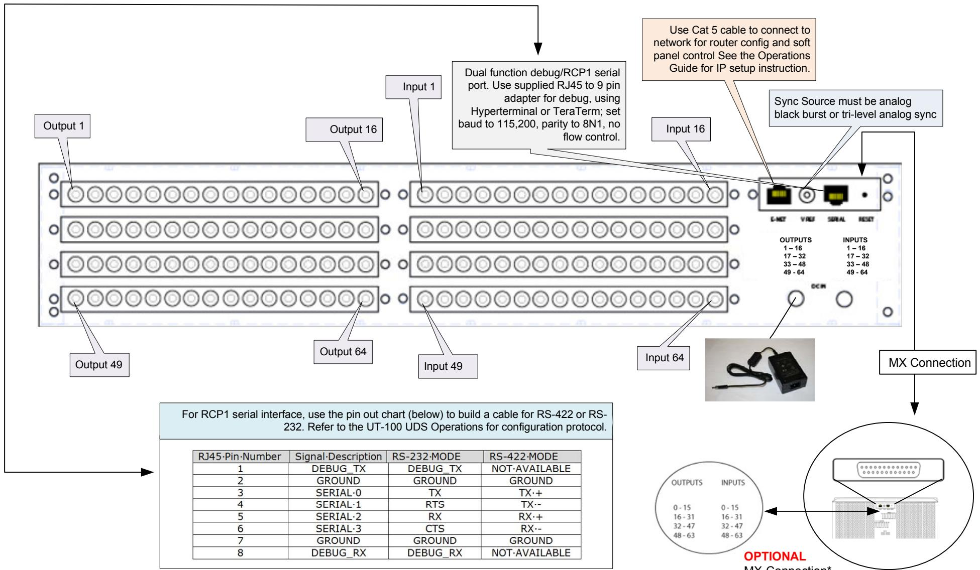
The MX configuration is offered as an option when tying the router to an SC-4 or SC-400 control system. The bubble callouts (above) illustrate the MX/ serial connection – installed when the MX configuration is ordered.
