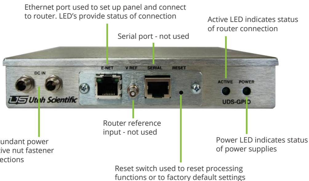
Ethernet port used to set up panel and connect to router. LED's provide status of connection
