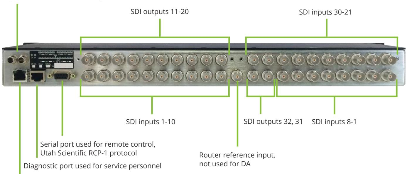
Ethernet port used to set up and control router, connect remote panels and remote control. Utah Scientific RCP-3 protocol. LED's provide status of connection.
