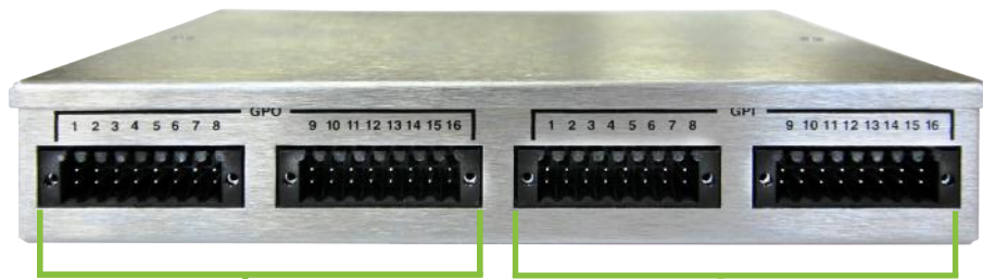
1-16 GPO's - Assignable to any source-destination combination
