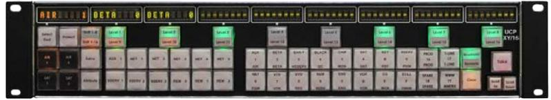
The UCP-XY/E is a full-matrix X-Y panel used to route any source to any destination, with full 16-level breakaway and status. The panel includes eight alphanumeric displays, each with eight characters, providing direct indication of status. A ninth display shows the active destination. The 20-button keypad provides the ability to select sources and destinations by name or numeric value. Scroll-up and scroll-down buttons provide easy navigation of sources and destinations.
