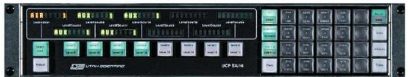
The UCP-SX/E is a full-matrix X-Y panel used to route any source to any destination, with full 16-level breakaway and status. The panel includes eight alphanumeric displays, each with eight characters, providing direct indication of status. A ninth display shows the active destination. The 20-button keypad provides the ability to select sources and destinations by name or numeric value. Dedicated salvo, attribute, and protect/lock output buttons are included.
