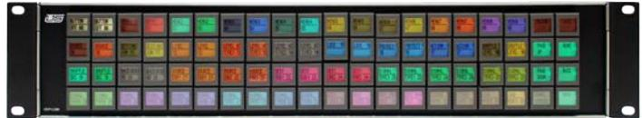
The UCP-LC80 panel offers two rows of programmable buttons with eight characters and user-definable colors. The flexible, 32-menu layering structure provides fast access to a variety of panel configurations. All buttons are fully programmable for any function such as source, destination, salvos, level mapping, audio attributes, protect/lock, paging, and breakaway switching.
