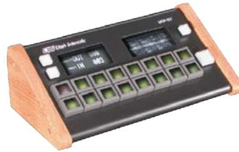
The UCP-DT/A/E is a desktop version of the UCP-MM/A full matrix X-Y panel, designed for placement on a desktop, console, or other location where rack-mount space is not available. The panel's two touch-screen LCD display panels offer highly legible read-out of levels, sources, destinations, or router status, and 16 selector buttons each provide an 8-character LCD display.
