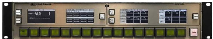
The UCP-MM/B/E is a full matrix X-Y panel used to route any source to any destination, with full, 16-level breakaway. The panel's four touchscreen LCD display panels offer highly legible read-out of levels, sources, destinations, or router status and 20 selector buttons.
