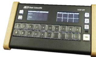
The UCP-DT/B/E is a desktop version of the UCP-MM/B full matrix X-Y panel, designed for placement on a desktop, console, or other location where rack-mount space is not available. The panel's two touch-screen LCD display panels offer highly legible read-out of levels, sources, destinations, or router status, and 20 selector buttons each provide an 8-character display.
