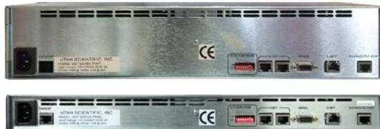
Flexible connection options include Ethernet or U-Net (Utah Scientific's network that enables serial looping of panels) using standard CAT-5 cabling. In critical applications, UCP panels provide unique redundancy by allowing both connection methods; in the event of an Ethernet or U-Net failure, the panel automatically switches to the alternate connection mode.
