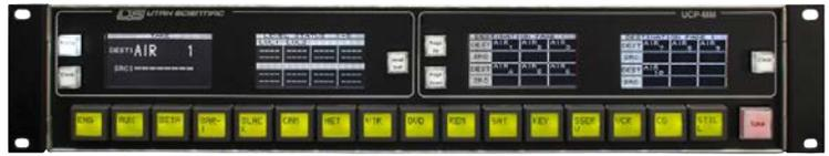
The UCP-MM/A/E is a full-matrix X-Y panel used to route any source to any destination, with full, 16-level breakaway. The panel's four touchscreen LCD display panels offer highly legible read-out of levels, sources, destinations, or router status, and the 16 selector buttons each have an eight-character LCD display.
