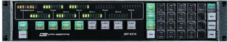
The UCP-MX/E is a full matrix XY panel used to route any source to any destination, with full 16-level breakaway and status. The panel includes eight alphanumeric displays, each with eight characters, providing direct indication of status. A ninth display shows the active destination. The 20-button keypad provides the ability to select sources and destinations by name or numeric value. Dedicated salvo, attribute, and protect/lock output buttons are included.
