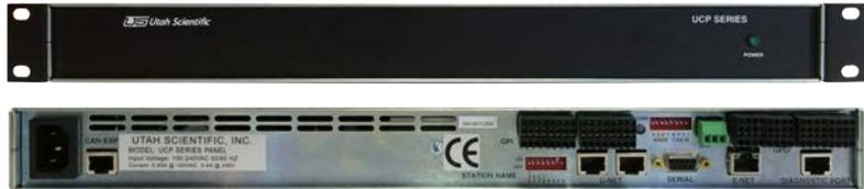
The UCP-GPIO/E provides the means to extend any Utah Scientific router control system to external devices by means of contact closures. The 16 in-bound contact closures (GPIs) are opto-isolated for ease of installation. These contacts can be configured for latching or momentary operation, and they are programmable for mapping the individual contacts to specific source-destination combinations.
