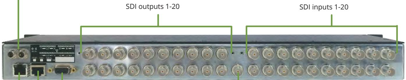
Serial port used for remote control, Utah Scientific RCP-1 protocol
