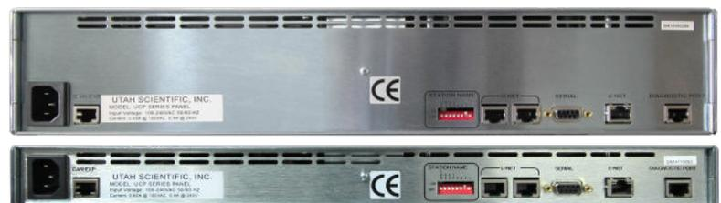
Flexible connection options include Ethernet or U-Net (Utah Scientific's network that enables serial looping of panels) using standard CAT-5 cabling. In critical applications, UCP panels provide unique redundancy by allowing both connection methods; in the event of an Ethernet or U-Net failure, the panel automatically switches to the alternate connection mode.
