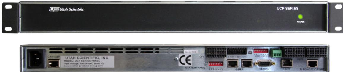
The UCP-GPIO/E provides the means to extend any Utah Scientific router control system to external devices by means of contact closures. The 16 in-bound contact closures (GPIs) are opto-isolated for ease of installation. These contacts can be configured for latching or momentary operation, and they are programmable for mapping the individual contacts to specific source-destination combinations.
