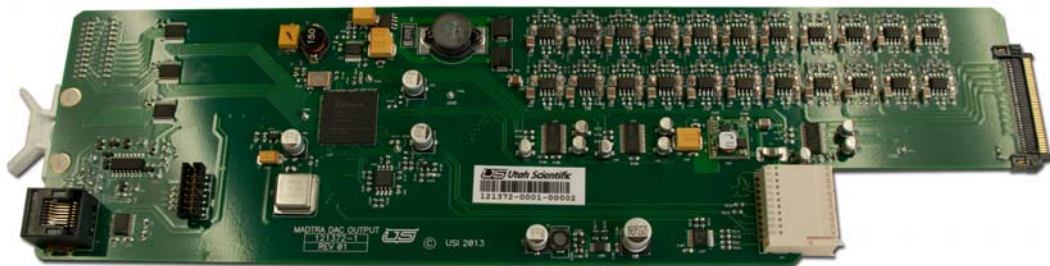
Figure 1-9. DAC Audio Output (121372-1)
