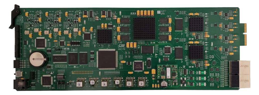
MC-402 card can be placed in any series 2 SDI router output slot with its accompanying rear panel.
