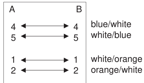
FIGURE 3-12. U-Net Cable Pairs and Pin-out
