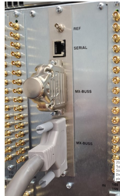
Figure 2: MX-Bus port view of UHD-288
